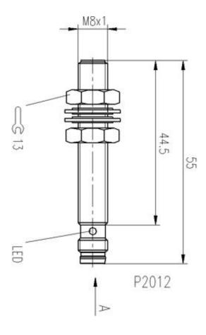
Inductive Sensors BES 516-377-S49-C M8x1 x 55 normally-closed Sn=1,5mm shielded
